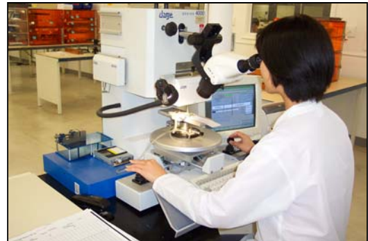
Destructive testing to ensure wire bond quality
